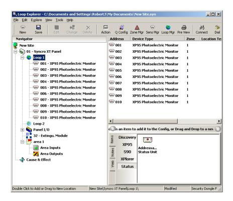
To change the address of the Status or Hold off unit, right click its icon and select device operations then change address from the drop down menus.
